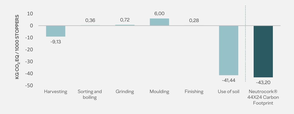
Neutrocork<sup>®</sup> carbon footprint, according to standard 14067:2018: **-43.20 kg CO2eq**/1000 stoppers.
