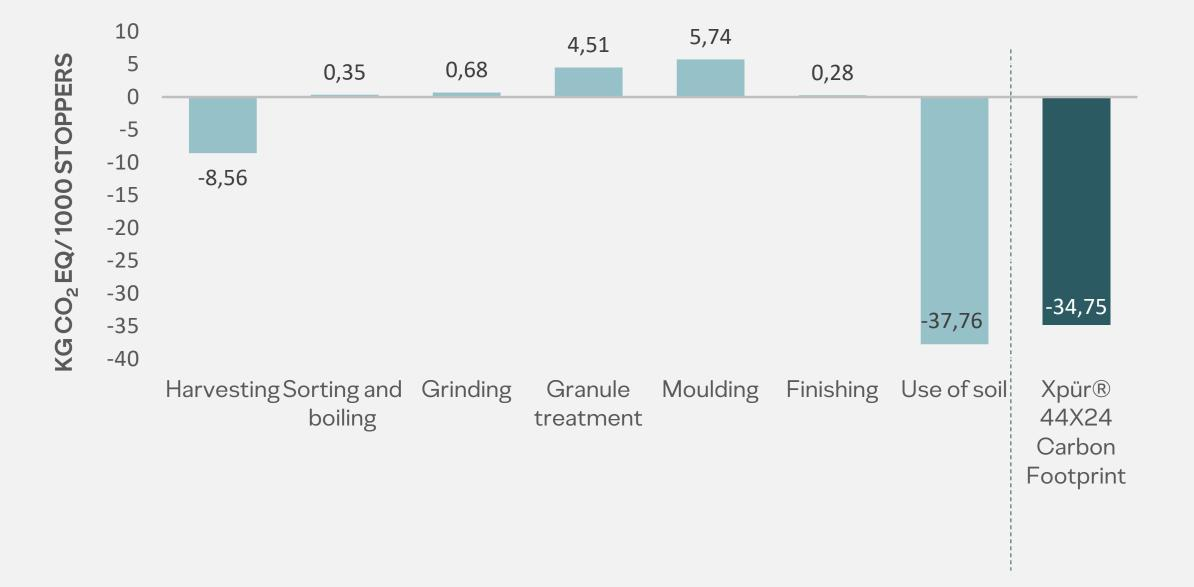
Xpür<sup>®</sup> carbon footprint, according to standard 14067:2018: -34.75 kg CO2eq/1000 stoppers.
